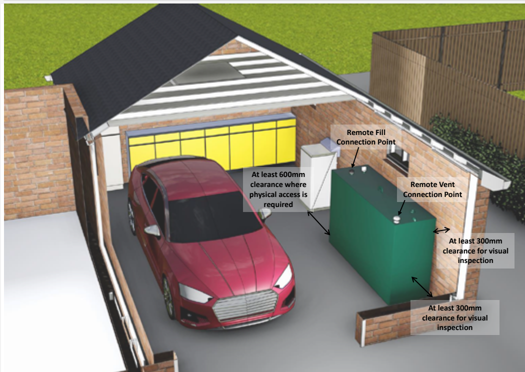
Typical internal 1 Hour fire rated Tuffa FP Tank installation:
